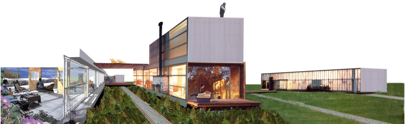
Image 7. Railway City, European 8. Runner-up award 2007 in Hamar, Norway. Mobile housing system consisting of two units: a based-space frame for living and a green house container performing as thermal buffer. Source: Suau archive.
